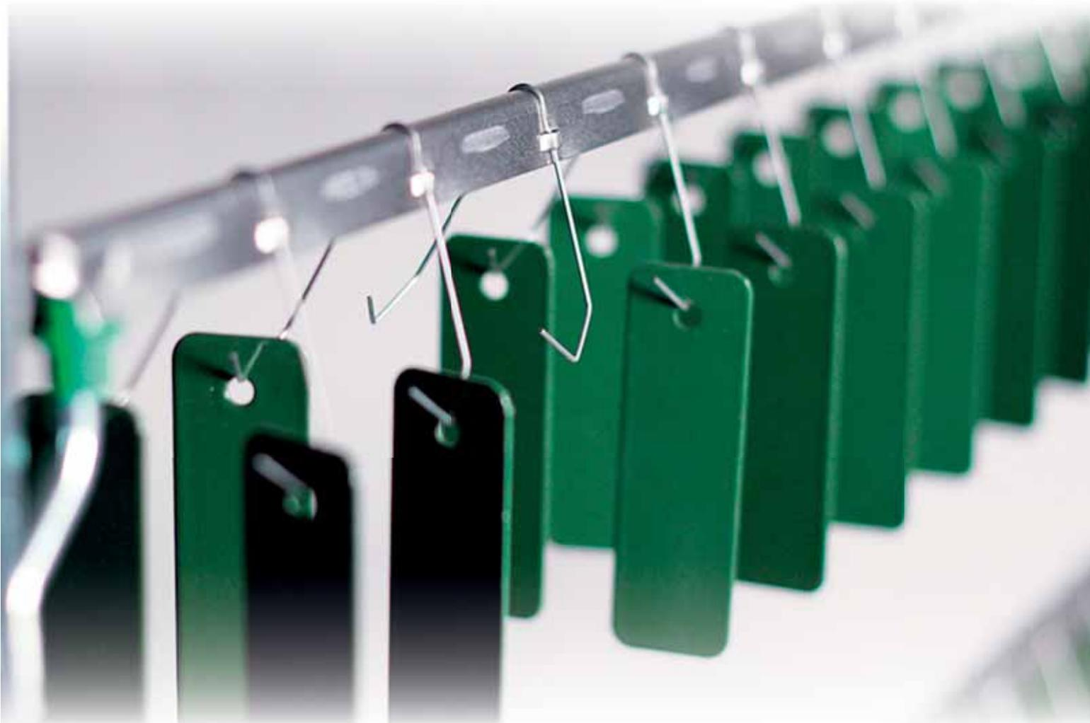
*Opening photo: the search for the optimal and most efficient method to hang the workpieces for the coating process is a crucial aspect for reducing the cost of the entire production process. The HangOn products, distributed in Italy by Tecno Supply, can help to achieve a higher production efficiency.*
